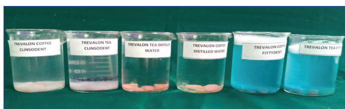
[Table/Fig-4]: Trevalon samples immersed in clinsodent, fittydent and distilled water.
