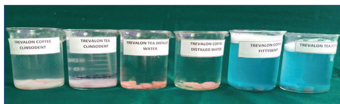
[Table/Fig-4]: Trevalon samples immersed in clinsodent, fittydent and distilled water.
